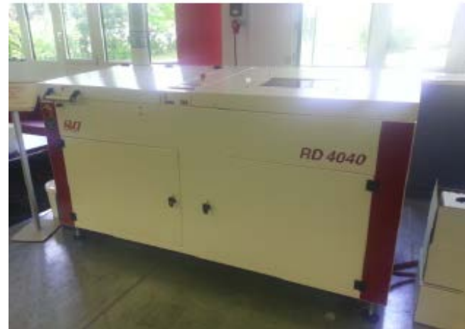
Figure 4. Vapor phase reflow machine – internal preheating.
