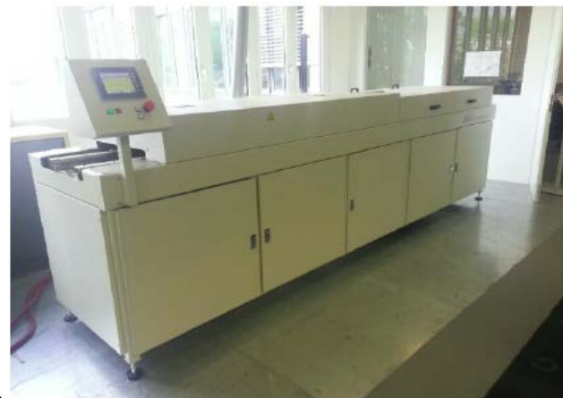
Figure 5. Vapor phase reflow machine with in-line convection preheating.
