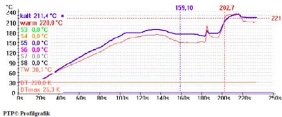
Figure 7. In-line inert convection preheat vapor phase reflow profile used for VP 2.
